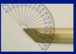
Angle between the secondary cutting edge and the tip (aka blunt spine) is less 90 degrees
