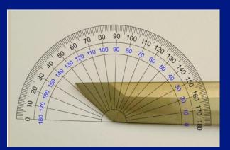
Angle between the cutting edges is over 90 degrees
